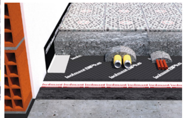
↑ Floating screed can also be created in single-layer solution. Isolmant UnderSpecial BiPlus is the ideal solution due to the presence of the fiber-reinforced anti-tear fabric.
